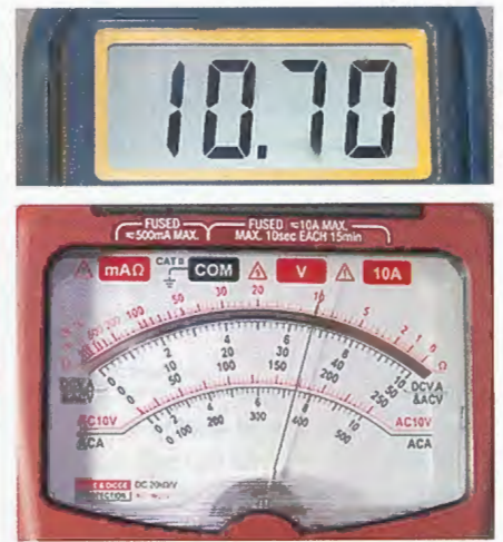
Photo 5: This shows the two meters measuring the same 10,000 ohm resistor. The digital meter shows 10.70 or 10,700 ohms. The analog meter's pointer is almost on the 10 mark using the X1K range.
