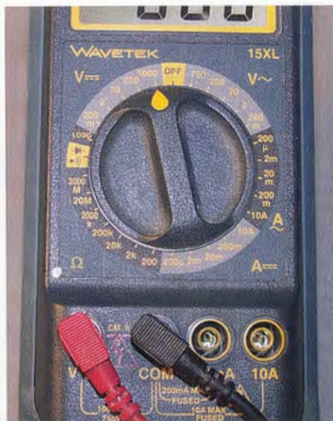
Photo 2: This is a close-up of the selection dial on the digital meter. It has five function ranges plus a diode/continuity test, a logic test where it can be used to test digital logic circuits and an off position. You will see that most of the range selections are multiples of 2 – i.e. 2, 20, 200. The actual maximum measurement is just less than 2 or 20 etc. For instance, on the 20-volt range, the maximum measurement is 19.99 volts. The highest D.C. and A.C. voltage ranges have different maximums.
