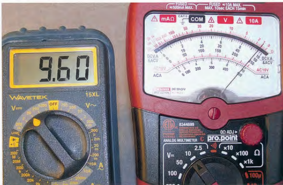
Photo 4: This shows both meters measuring the voltage of a fresh 9-volt battery. The digital meter shows 9.60 volts. The analog meter is using the 0, 2, 4, 6, 8, 10 scale. The odd number values are designated by a thicker mark between the even numbers. The smallest divisions represent two volts. You can see that the pointer is right on the 9.6-volt mark. It's just a matter of counting the marks: number 8, big mark 9, little marks 2, 4, 6 giving you 9.6 volts.
