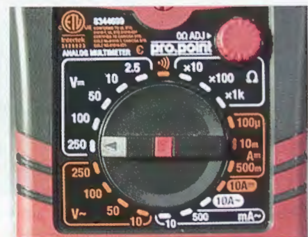
Photo 3: This is a close-up of the analog meter's dial and face. Unlike the digital meter, the ranges don't follow a pattern of multiples of 2. If you compare the ranges to the maximum numbers on each of the meter's scales, you will see how they match up. The scales require some interpretation as you read them. For instance, if you are using the 10 V.D.C. range, you will read the black scale marked 0, 2, 4, 6, 8, 10. If you are using the 100 V.D.C. range, you will use the same scale, but now you multiply the reading by 10 so that they now become 0, 20, 40, 60, 80, 100. The D.C.V. scale that goes from 0 to 50 is used for both the 5-volt and the 50-volt ranges. There are separate scales for 10 V.A.C. and A.C. amps.
