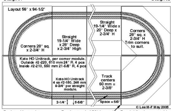
Designed for easier storage & transport. Track extends 1/32" beyond each end for positive locking. Two folding banquet tables 30" x 8' hold this layout.
